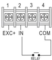
Relay Contact: NPN 0~400 Hz
